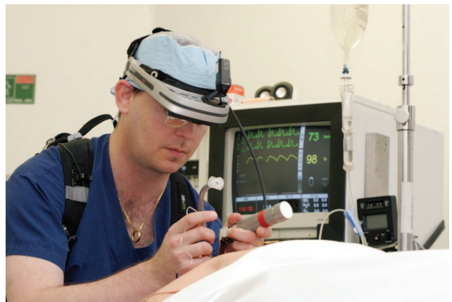
Figure 1. An anesthesiologist intubates a mannequin while monitoring with a head-mounted display (HMD) in Experiment 1. The HMD projects a subset of the vital signs presented on the patient monitor into the anesthesiologist's field of view (Fig. 2). The simulated patient monitor (in the background) includes waveforms (electrocardiogram, SpO 2 , and CO 2 ) and numerical vital signs (heart rate, SpO 2 , ETCO 2 , noninvasive arterial blood pressure (NIBP), temperature, and end-tidal/inspired: agent, N 2 O and O 2 ).
