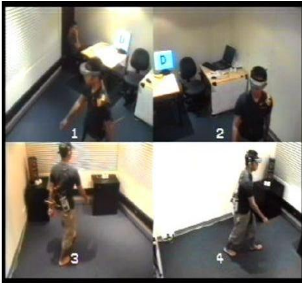
Figure 2. Quad display of a participant during the experiment. Participant is wearing the HMD and earpiece and is walking towards a pushbutton. Pushbuttons were located in each corner of the room. Letter “D” in frame 2 is a visual stimulus telling the participant which button-box to push.
