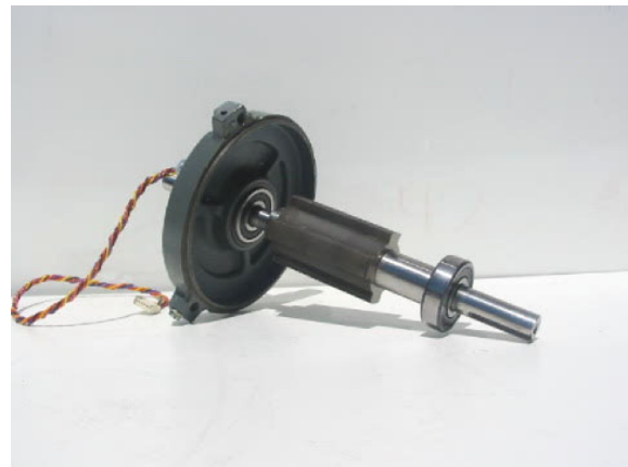
Figure 7: Rotor and shaft.
