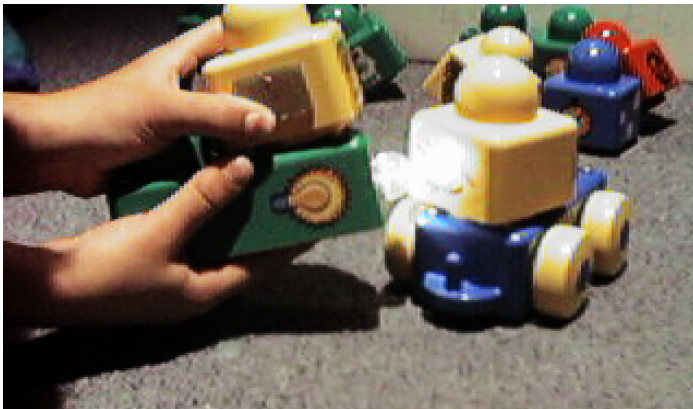
Figure 4: A remote control car demonstrates interaction between block stacks. The touch block on the light block forms the remote control for the car formed by placing a seeing block on a movement block.
