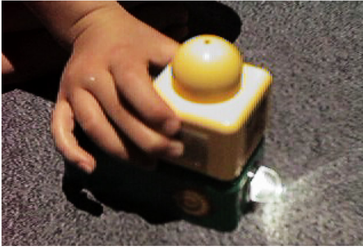
Figure 2: A touch block attached to a light block will cause the light to turn on whenever the sensor plate is touched.
