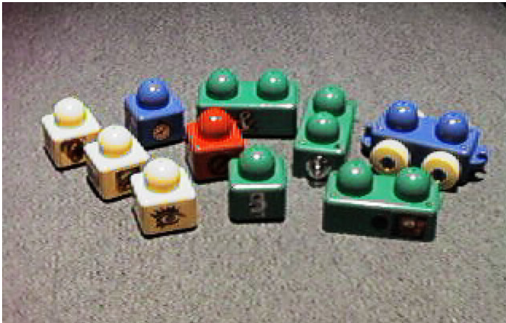
Figure 1: The complete Electronic Block family: the three sensor blocks are to the left, the four logic blocks are in the centre, and the action blocks to the right.
