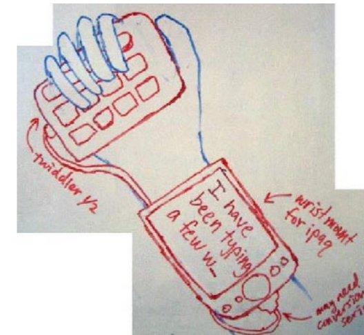
Figure 1: A low-fidelity prototype of a mobile data logger with a chord keyboard
