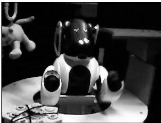
Fig. 1. The Task Environment. An AIBO ERS-7 is mounted on a swivel chair surrounded by a hanging toy, a bitable piece of foam and a “Dora the Explorer” musical toy that it can learn to interact with.
