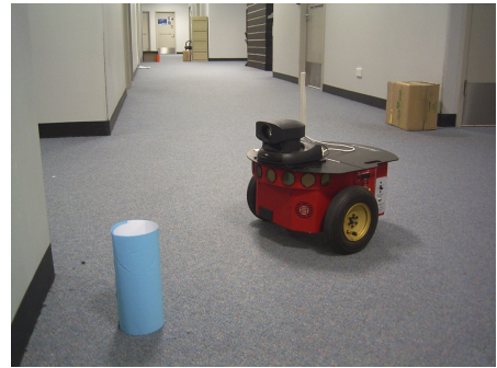
Figure 5. Testing arena and Pioneer robot. The Pioneer is equipped with a ccd camera, wheel encoders and eight sonar sensors spread over the front half of the robot. Coloured cylinders are used as artificial landmarks.
