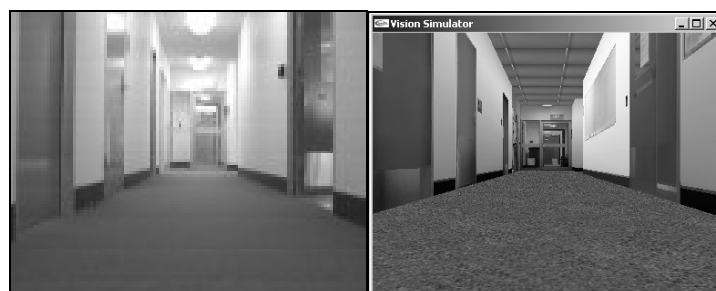
Figure 2 The robot's world comprises halls and open plan offices. A simulated world has been built to mirror the real world. The features of the environment shown in the visual images seen by the robot include the floor, walls, desks, chairs, and filing cabinets. The left image is from the robot's camera and the right image is the same location in the simulated world.
