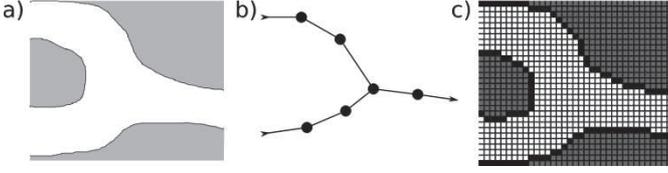
Fig. 3 RatSLAM and Gmapping use fundamentally different representations of their environment a) a junction where three paths meet b) the RatSLAM representation uses experiences connected by links. c) the Gmapping representation uses an occupancy grid where white indicates free space, black indicates an obstacle and grey indicates unknown.
