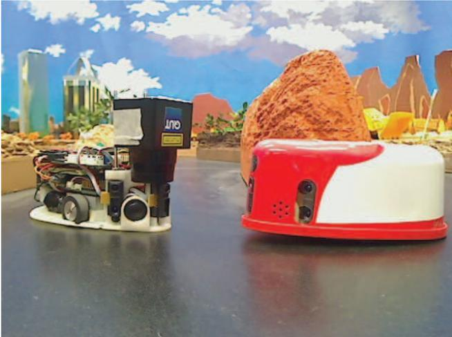
Fig. 1. Lingodroid iRats in conversation. On the right is a standard ‘camera iRat’ which has a forward facing camera inside the dot of the ‘i’. On the left is the modified ‘laser iRat’ which has a laser scanner mounted upside down. The standard iRat’s cover has been removed to fit the laser scanner. The two iRats are shown in the environment used for the studies in the paper (also see Fig. 2).
