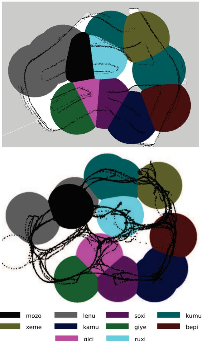
Fig. 4. Maps and Toponymic Lexicons developed for the laser iRat (top) and the camera iRat (bottom). The maps of both robots are recognizably the environment shown in Fig. 2, with a high degree of similarity between the locations for all of the toponyms.
