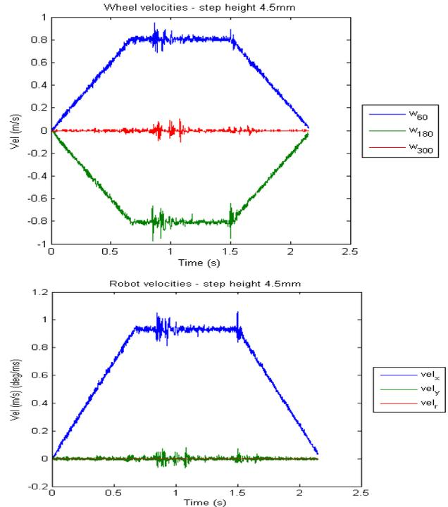
Fig. 9. Step height experiment with the spherical robot showing (top) wheel encoder velocities, and (bottom) the robot's velocity, transformed from the wheel encoder measurements. The graph shows the high amplitude oscillation that occurs as the wheel hits the edges.
