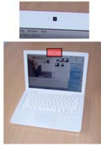
Figure 1 – Built-in iSight video camera on Apple Macbook . This camera was the sole source of sensory information for all experiments. The laptop was mounted on a chair for the indoor experiments and on a car for the outdoor experiments.
