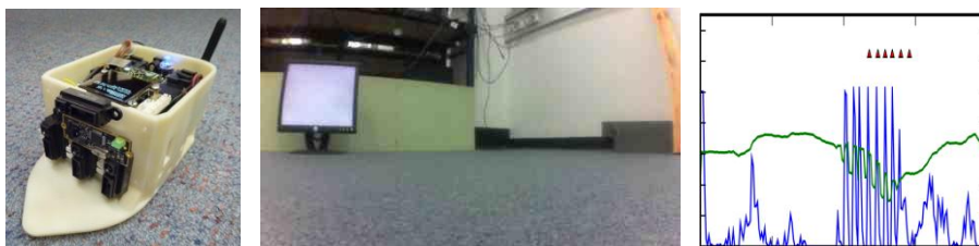
Fig 1. The rat animat and temporal dynamics of its visual environment. The rat animat (left, photo source [18]) moves autonomously through its office environment (typical camera view, centre). The average ambient light levels were recorded while the rat animat rotated 360 deg (right, green trace). With high gain the signal derivative shows fast oscillations (blue trace). A monitor flashing at 1 Hz superimposed an additional dynamic on the ambient light, and could be seen for 110 degrees.
